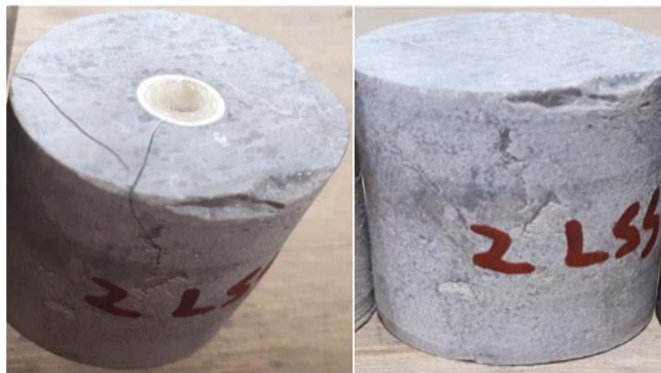
Fig. 3 Right) Intact Limestone dry sample. Left) Lased Carbonate dry sample under Pressure.
